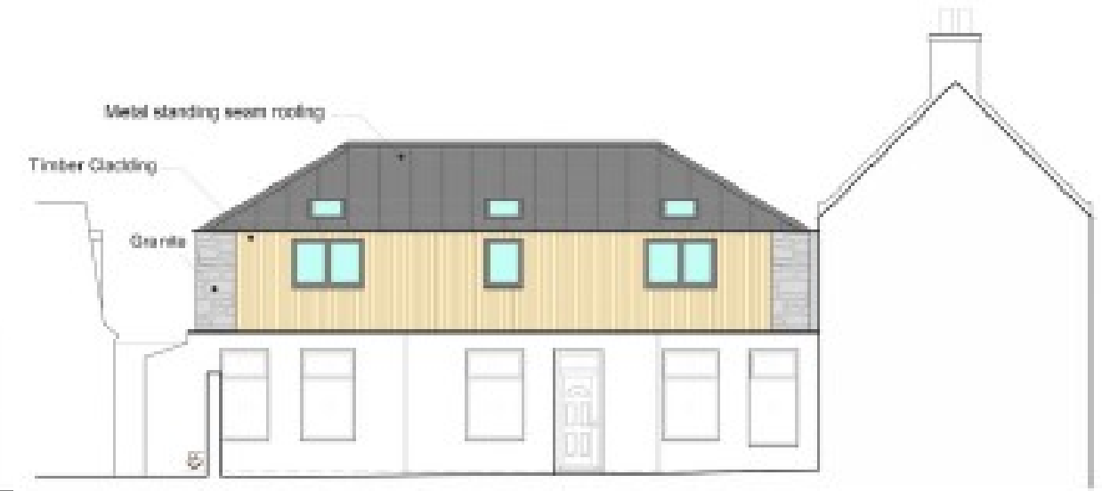
South West Elevation - 1:100
